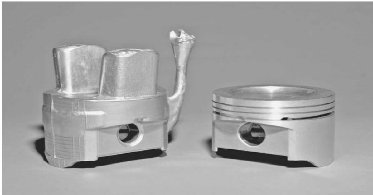
Figure 18 : Aluminum piston for an internal combustion engine: (a) as cast and (b) after machining. The part on the left is as cast, including risers, sprue, and well, as well as a machining allowance; the part on the right is the piston after machining.
